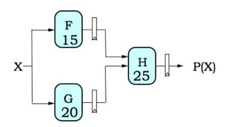
Unpipelined: L = 45ns, T = 1/L = 1/(45ns)2-stage pipeline [ $t_{CLK}=25ns$ ]: L = 2\*25 = 50 ns, T = 1/(25ns)
