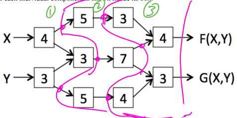
(A) Using ideal zero-delay registers, mark the location of the minimal number of registers necessary to achieve maximum throughput. Give the latency and throughput of your pipelined circuit.
