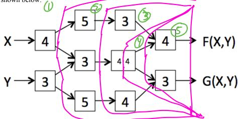
(B) Using ideal zero-delay registers, mark the location of the minimal number of registers necessary to achieve maximum throughput. Give the latency and throughput of your pipelined circuit.
