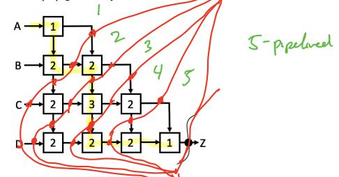
(A) Please pipeline the circuit above for maximum throughput with the minimum possible latency using ideal pipeline registers ( $t_{PD} = 0$ ,  $t_{SETUP} = 0$ ). Show the location of pipeline registers in the diagram above using filled-in circles, like the one shown on the Z output. Please give the latency and throughput of the resulting pipelined circuit.
