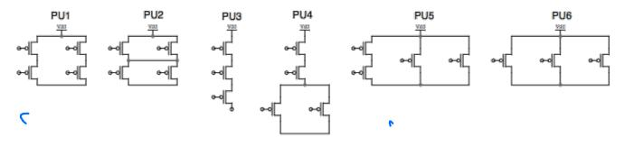
You can connect one of the inputs (A, B, C, or D) or a constant (GND, or VDD) to each pFET, allowing these pullups to be used in various ways to build gates with various numbers of inputs. Your goal, however, is to select the pullup that uses the minimum number of active transistors for each of the gates you are designing (i.e., a pFET that is never on is *not active*).
